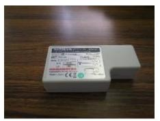
Figure 17. High-dose CsI detector (Hamamatsu Photonics C12137)
