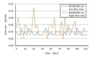
Figure 19. Measured value dispersion check
