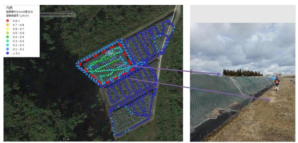
Fig. 5.4. Combination of UAV (marked within red rectangle) and backpack based radiological mapping, carried out at one of the temporary storage sites of the Fukushima Prefecture. Image: Fukushima Prefecture.
