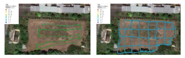
Fig. 5.2. Example of in-situ measurements (not-corrected raw data) performed in the area accessible both for backpack and UAV techniques: data points obtained with the UAV system (Geiger-Müller counter) flying at 10m altitude (on the left); data points obtained with backpack system (CsI spectrometer) walking throughout the area with the detector located at 1m altitude (on the right). Image: Fukushima Prefecture.
