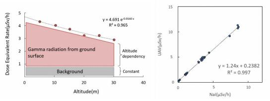
Fig. 5.3. On the left: illustration of exponential dependence of the dose equivalent rates measured by the UAV-based system and represented as a function of altitude. On the right: illustration of linear dependence of UAV data obtained with Geiger-Müller counter with respect to reference NaI data (both measurements were performed at 1 m altitude and for different dose equivalent rates). Image: Fukushima Prefecture.
